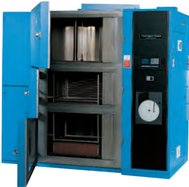
A Double Duty Thermal Shock increases throughput by making double use of the center cold zone. A two-tiered transfer basket shifts one product load from hot to cold while the other product load shifts from cold to hot.
