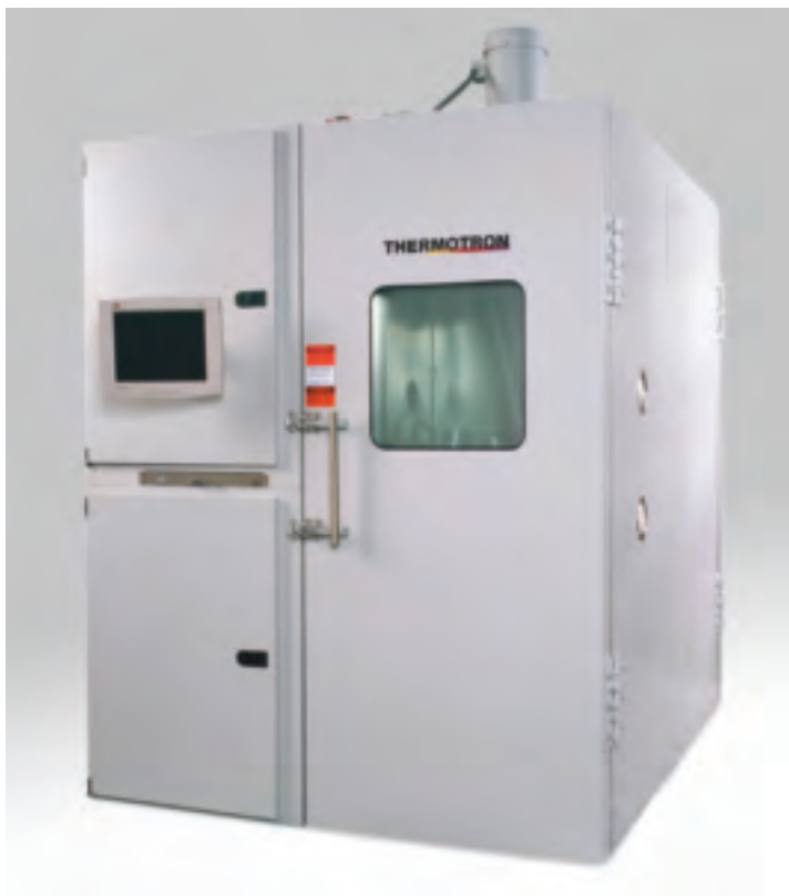
The AST-20R uses mechanical refrigeration instead of liquid nitrogen to achieve rapid cooling rates required for HALT and HASS testing. By using mechanical refrigeration, installation and operating costs are reduced.
