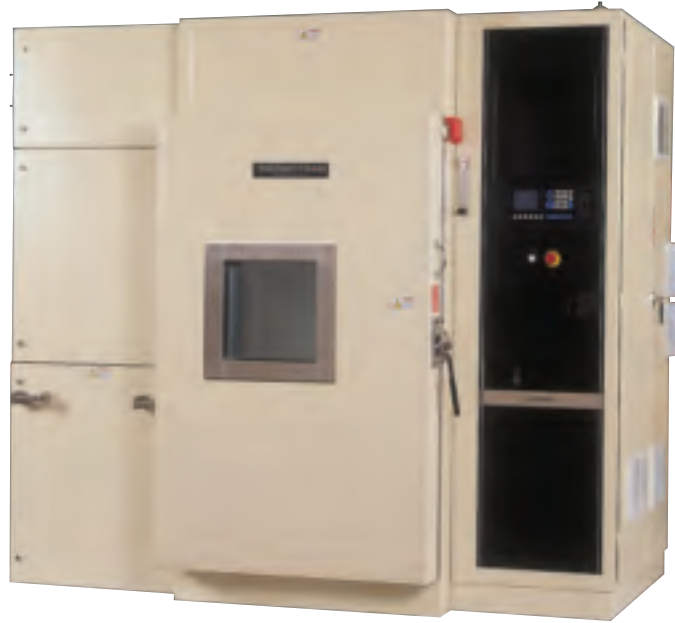
ESS Chambers expose product flaws and eliminate infancy failures.
