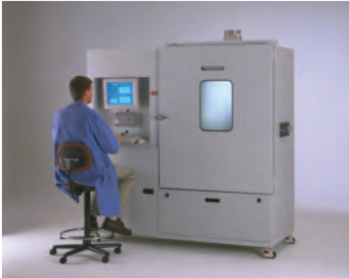
AST quickly forces failures through rapid product temperature change rates and aggressive repetitive shock vibration. AST chambers are available in various sizes, including AST-8 (pictured above), AST-35 and AST-70.
