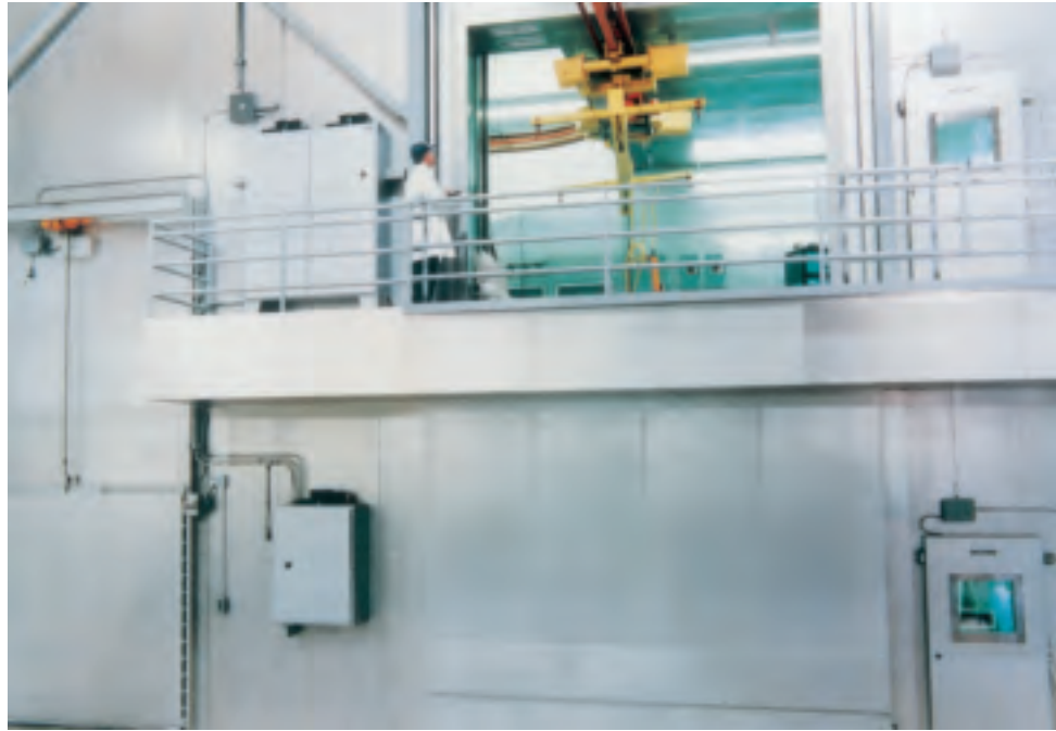
This 33,600 cubic foot Psychrometric Test Facility was developed for a major HVAC manufacturer of air conditioners and heat pumps. It supports 24 hour per day automatic operation, reduced set-up time, and improved accuracy and test repeatability.
