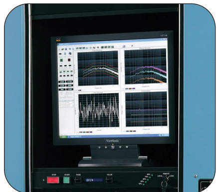
above: Close-up of Thermotron's vibration controller located in the console.
