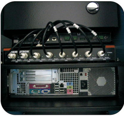
above: Thermotron's VIO module box, part of the vibration control system.
